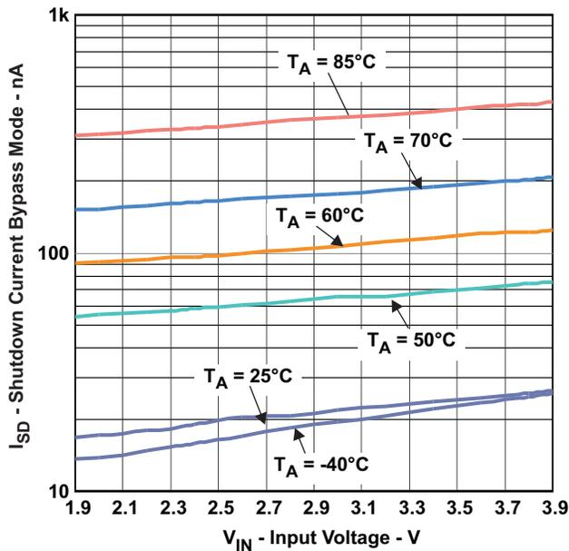
Figure 5. Shutdown Current Bypass Mode vs Input Voltage
