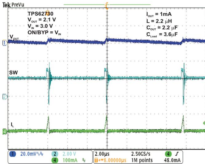
Figure 17. DC/DC Mode Operation  $I_{OUT} = 1\text{ mA}$
