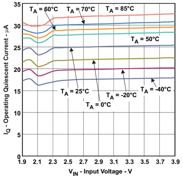
Figure 6. Operating Quiescent Current vs Input Voltage
