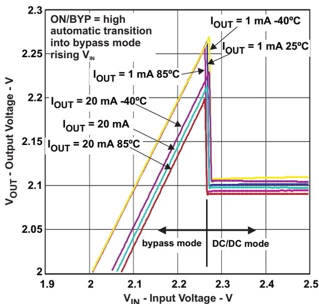
Figure 11. Automatic Transition into Bypass Mode - Rising  $V_{IN}$
