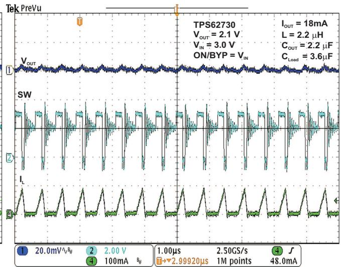
Figure 18. DC/DC Mode Operation  $I_{OUT} = 18\text{ mA}$
