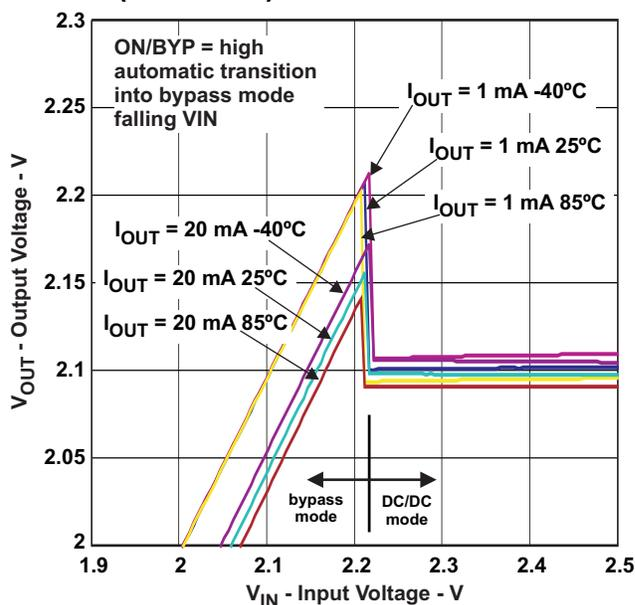
Figure 10. Automatic Transition into Bypass Mode - Falling  $V_{IN}$
