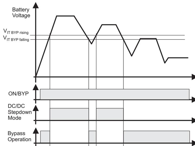
Figure 28. Operation Mode Diagram with ON/BYP = High
