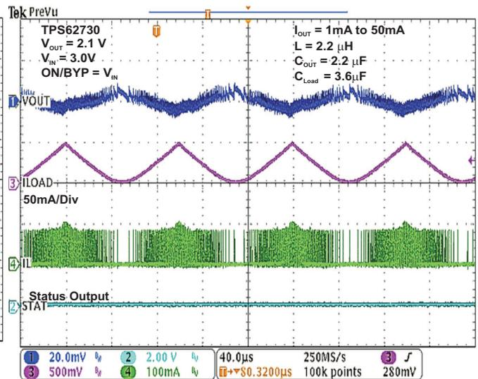
Figure 22. DC/DC Mode  $V_{OUT}$  AC Load Regulation Performance
