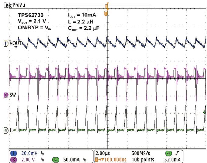
Figure 16. DC/DC Mode Operation  $I_{OUT} = 10\text{mA}$
