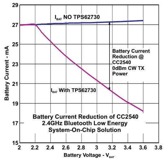
Figure 26. Battery Current Reduction vs Battery Voltage
