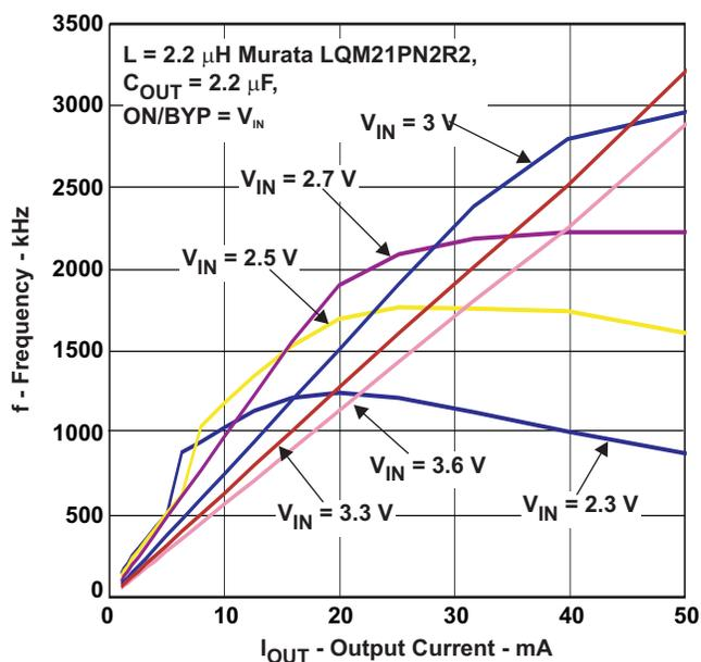
Figure 12. Switching Frequency vs  $I_{OUT}$  vs  $V_{IN}$
