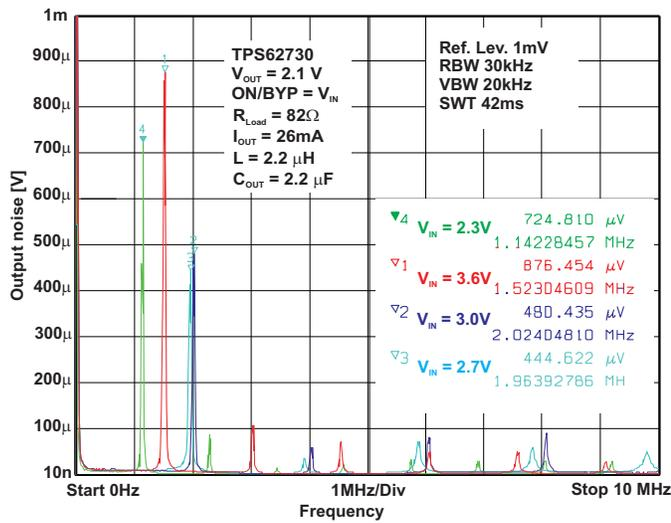
Figure 25. Spurious Output Noise TPS62730 I<sub>OUT</sub> 26mA
