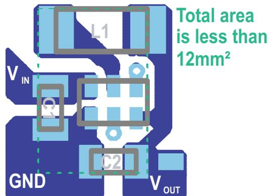
**Figure 33. Recommended PCB Layout for TPS62730**
