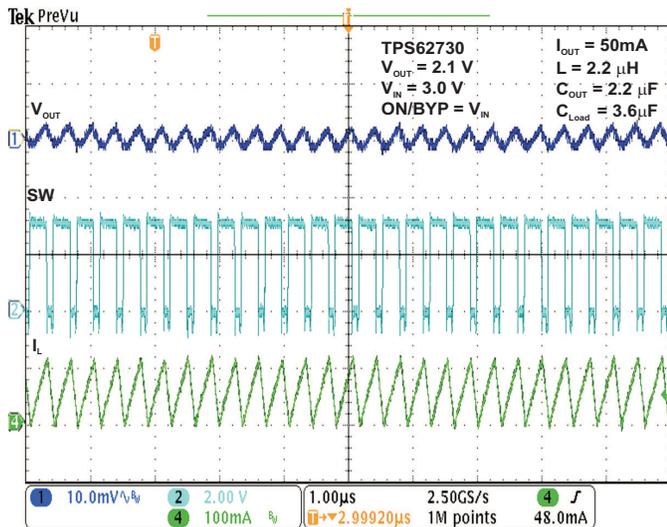
Figure 19. DC/DC Mode Operation  $I_{OUT} = 50\text{ mA}$
