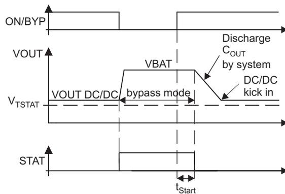
Figure 29. Signal Status Diagram ON/BYP, VOUT, STAT
